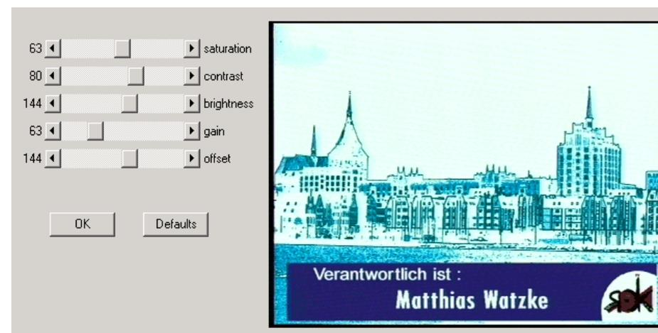
position of the gain slider has an influence on the image. Gain adjustment has an effect similar to contrast adjustment, but a gain change appears in the analog video signal before it is digitized. This has a great advantage for further processing because it keeps all 256 grey levels.
